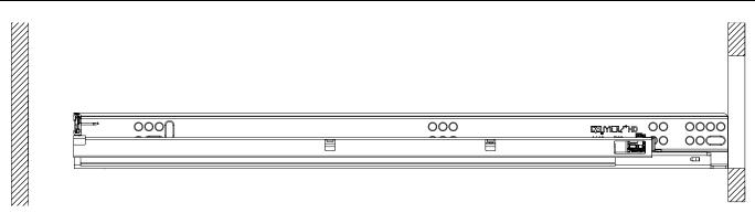
Min. Interior Depth Min. = Slide Length + Setback + 1/4" [6mm]
