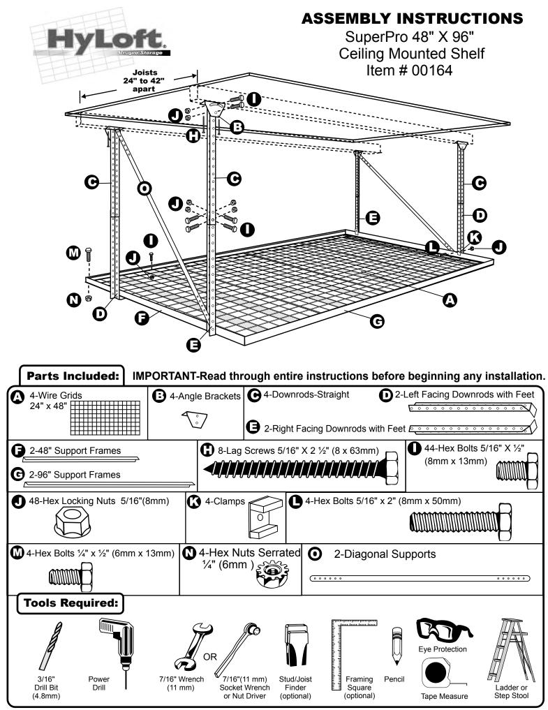
Identify and organize all parts before beginning installation. If any parts are missing, contact Knape & Vogt at 1-800-253-1561.
