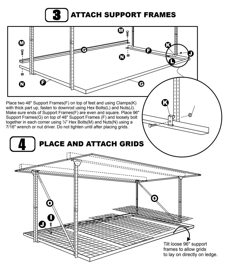
Lay 4 Wire Grids(A) evenly on 96" Support Frames with grid stiffeners on the underside. Tilt loose 96" Support Frames if necessary. Tighten bolts in each corner of support frames using  $\frac{1}{4}$ " Hex Bolts(M) and Nuts(N) wth a 7/16" wrench or nut driver. Fasten Wire Grids(A) as shown using 4 Hex Bolts(I) and Hex Nuts(J) for each grid.
