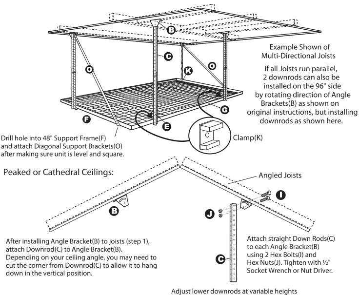
Adjust lower downrods at variable heights if needed so that Support Frames(F&G) will be level when installed. Continue with Steps 3 & 4.
