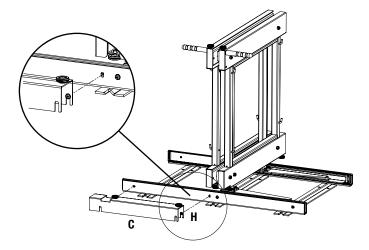
Set front guide stop (C) height to allow for proper roller clearance and operation.
