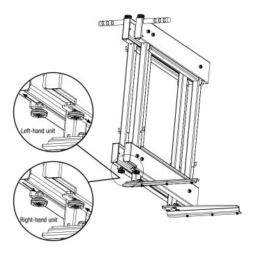
Attach center assembly (A) with feet to the slide base (E) with 6 - M5 x 8mm (G) screws.
