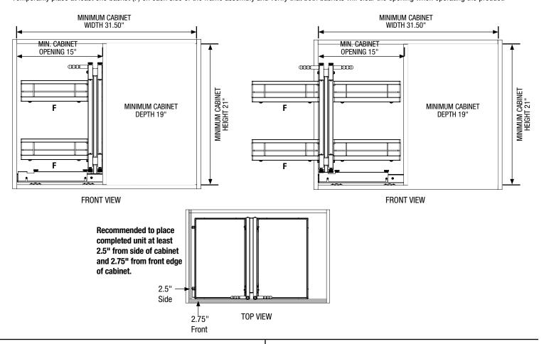
Once final position and proper clearances are confirmed, remove the baskets and install bottom frame to the base cabinet with 12 - ST4 x 14 (I) wood screws through the mounting brackets into the cabinet base.
