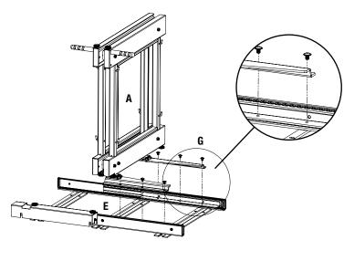
Attach front guide stop channel (C), replacing 2 - short M4 screws with 2 - longer M4 x 8mm (H) screws.
