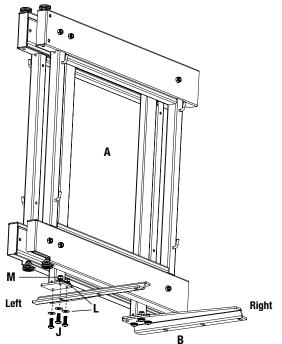
IMPORTANT: Before tightening fasteners holding support feet to sliding assembly, make sure feet are squared to sliding assembly.
