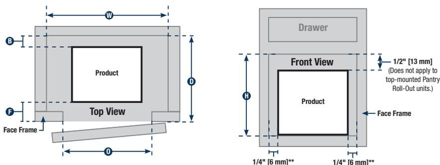
\* Minimum Cabinet Opening Width AND Minimum Cabinet Interior Width equals total width of completely assembled unit with all baskets applied, plus 1/2" clearance per side (1" total clearance for center-mounted units, 1/2" side clearance for side-mounted units). Dimensions shown are recommended minimum cabinet dimensions and clearances.
