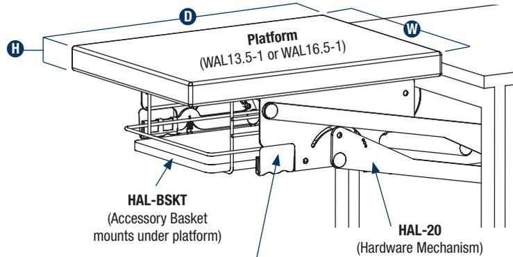
Pull up on right and left mechanism handles to unlock and lower Appliance Lift
