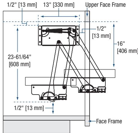
NOTE: Install 1/2" down and 1/2" back from upper Face Frame (as shown)
