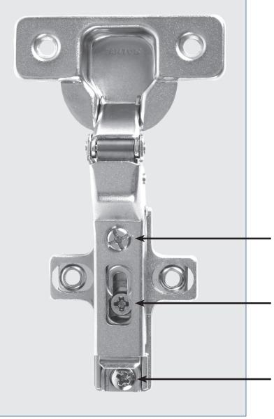
The Knape and Vogt Salice Hinge Kit program features three adjustable camms - horizontal (lateral), depth and vertical (height).
