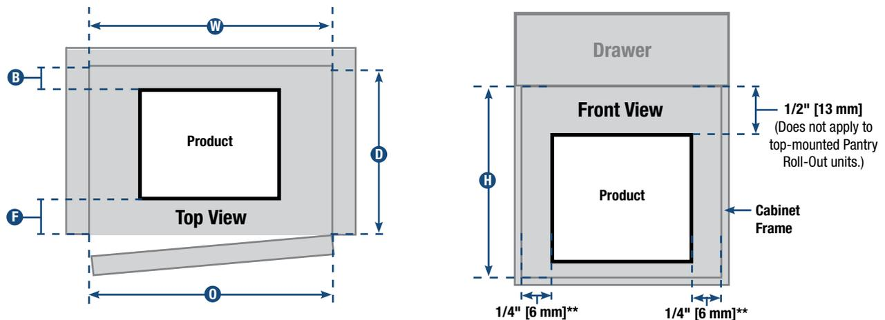
\*\* Slide-out Base Blind Corner Units and Base Cabinet Organizers require 1/2" side clearance on one side, not both.
