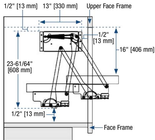
NOTE: Install 1/2" down and 1/2" back from Upper Face Frame (as shown)
