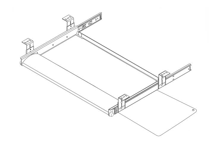
Note: Brackets mount in outboard position under work surface for application widths 24" or greater, and in the inboard position for widths less than 24"
