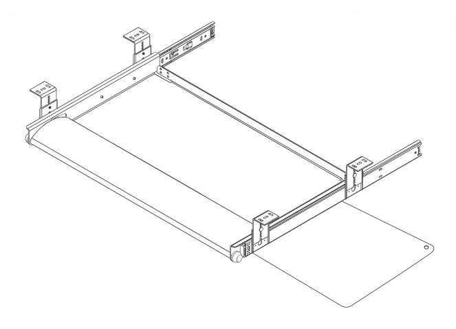
Note: Brackets mount in outboard position under work surface for application widths 24" or greater, and in the inboard position for widths less than 24"
