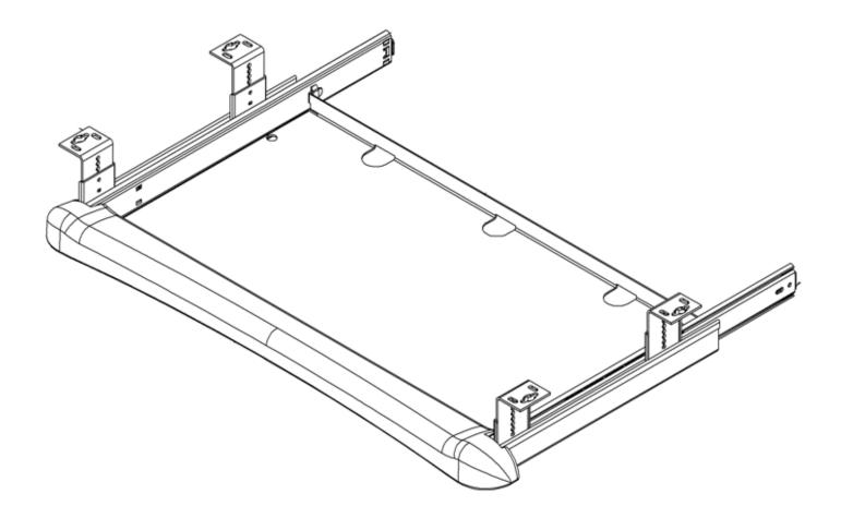
Note: Brackets mount in outboard position under work surface for application widths 23" or greater, and in the inboard position for widths less than 20.75"
