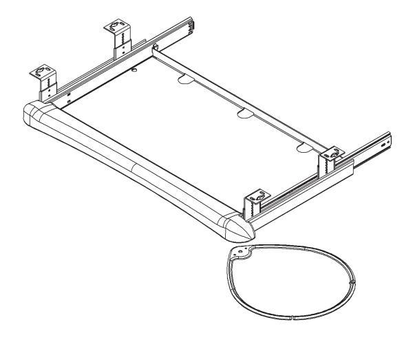
Note: Brackets mount in outboard position under work surface for application widths 23" or greater, and in the inboard position for widths less than 20.75"
