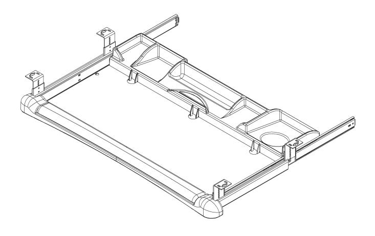
Note: Brackets mount in outboard position under work surface for application widths 29" or greater, and in the inboard position for widths less than 26.75"
