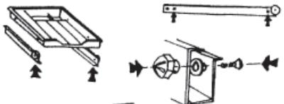
**4** Remove drawer from cabinet. Using a sabre saw and eye protection, remove the top portion of the back of the cabinet drawer so that it is no more than 1" high on the inside, and as wide as the lower tray.
