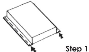
**2** Locate two drawer slide pieces stamped CL and CR. These are for bottom tray. Place tray with open end toward you. Place slide members with rollers on end nearest to you. Secure to bottom tray with 4 flathead screws and hex nuts through pre-drilled holes nearest the wings. Nuts go to outside of tray. Use the 2nd hole from each end of slides.
