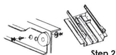
**3** Locate front of top tray (notched end). Slide members should be installed with flange up and rollers toward front of tray. Secure thru predrilled holes with four #6-32x1/4" flathead screws and 4 acorn nuts. Place a #8 washer between slide member and tray on right side only.
